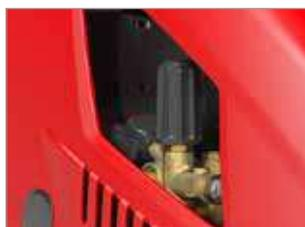
POMPA A.P. CON SISTEMA BIELLA MANOVELLA TESTATA IN OTTONE E PISTONI IN CERAMICA, VALVOLA AZZERAMENTO REGOLABILE.
